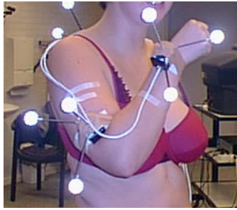
Figure 3: Attachment of Vicon markers and inertial sensing units to the forearm and upperarm. Sensors are adhered to the segment using double sided adhesive tape and secured using Leukoplast.
