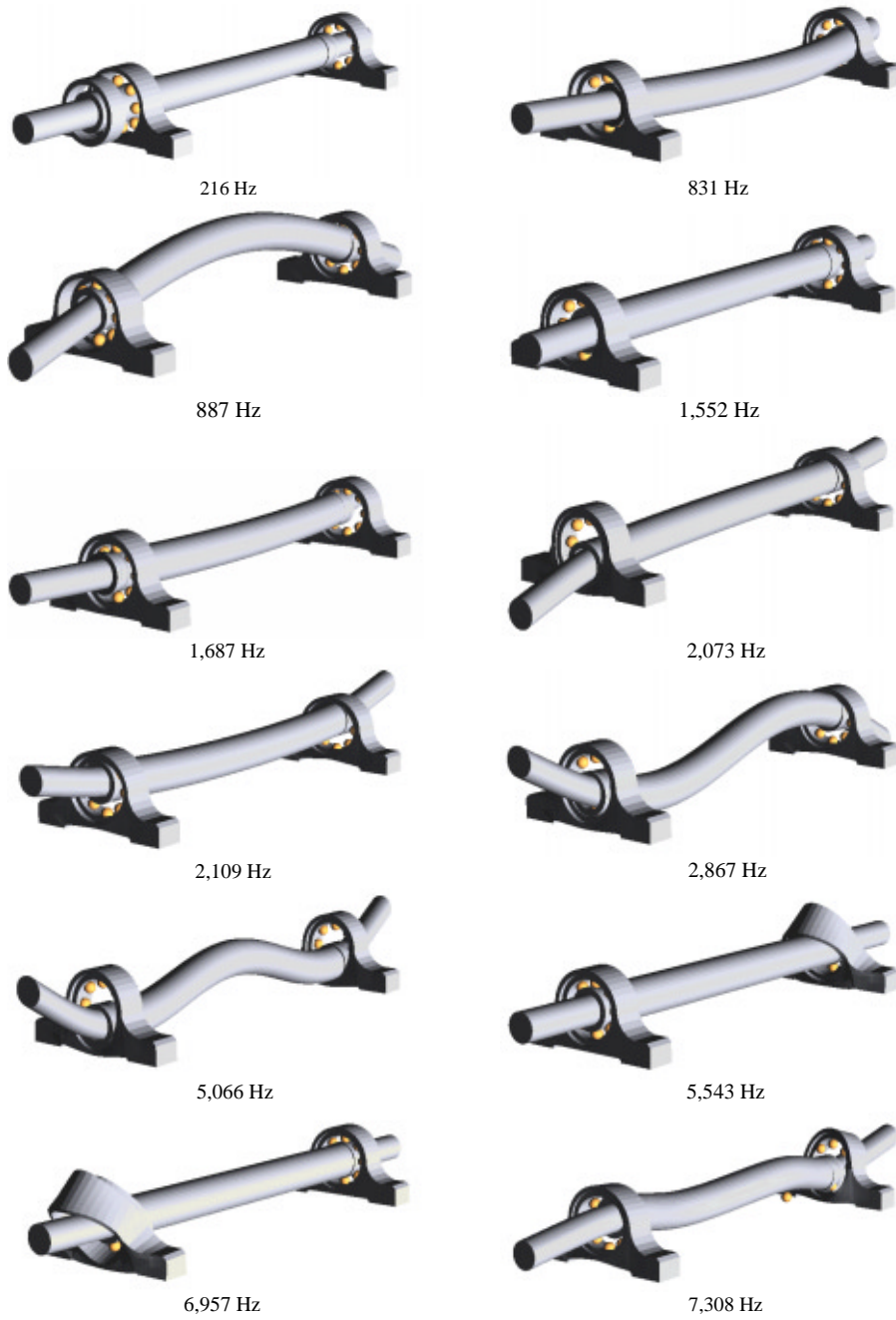
Figure 7.3: A number of important normal modes of the application.
