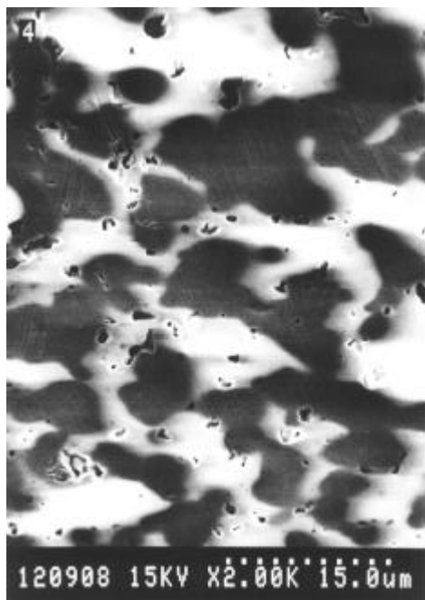
Figure 8.1. SEM picture of polished fresh BE25Ag40 membrane surface.
