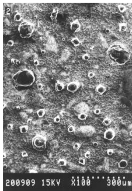
Figure 8.2. SEM picture of BE25Ag40 surface after thermal treatment at 993 K.
