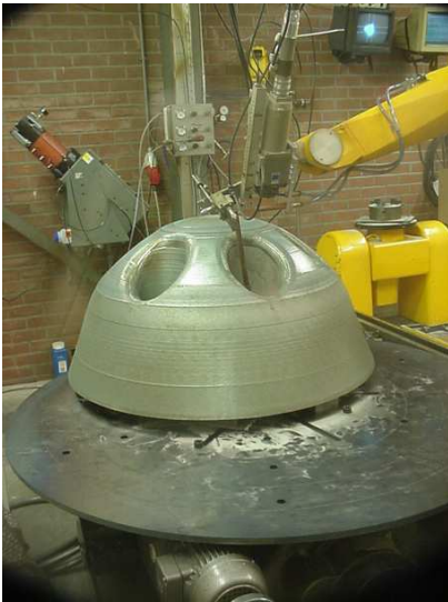
Figure 2.7: Cladding of a large heat exchanger kalott. Operational temperature > 1000^{\circ}\text{C} ( Courtesy of NedClad Technology BV).
