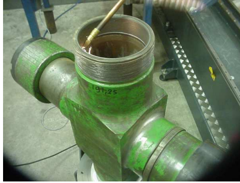
Figure 2.8: Cladding of a large valve ( Courtesy of NedClad Technology BV).
