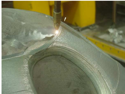
Figure 2.7: Cladding of a large heat exchanger kalott. Operational temperature > 1000^{\circ}\text{C} ( Courtesy of NedClad Technology BV).
