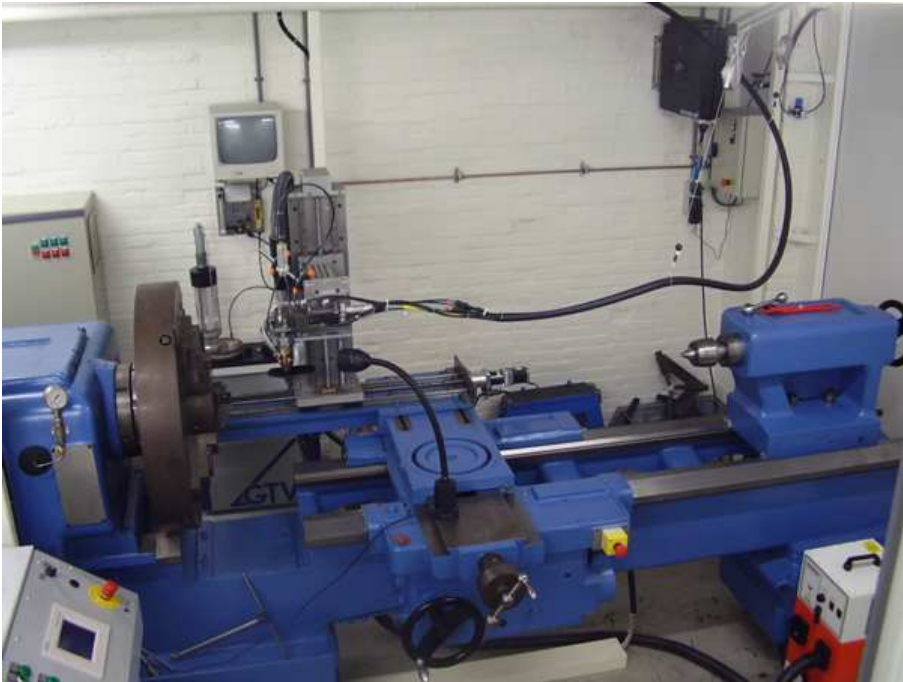
Figure 10.1: Cladding setup of SG&S using a turn table.
