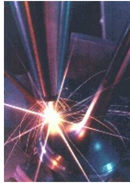
Figure 2.6: Laser cladding of a diesel engine intake valve.
