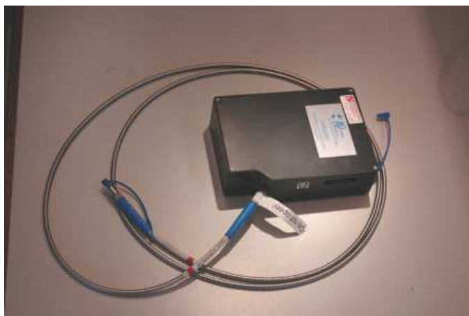
Figure 5.4: Photo of the Ocean Optics HR4000 spectroscopy with measurement fiber.
