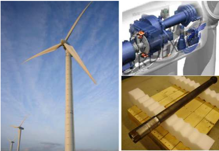
Figure 10.18: Windmill pitch shaft.
