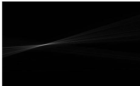
Figure 4.35: Hough transform for r(\phi) . Resolution of 0.1 degrees from -10 degrees to 10 degrees.
