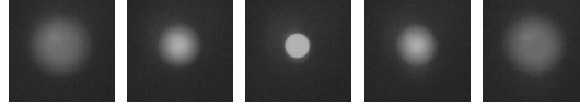
Figure 4.7: Sequence of images with the laser head moving from 3 mm below to 3 mm above the pilot focus
