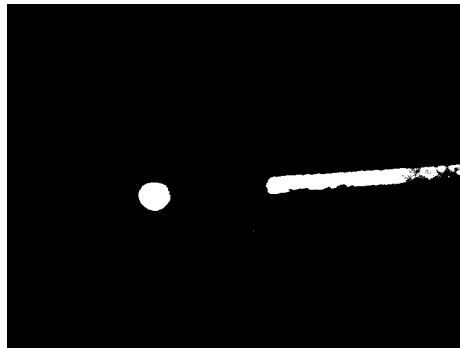
Figure 4.32: Thresholded camera image for combined tool calibration. Threshold value of 60
