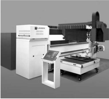
(a) Five-axis gantry robot. Courtesy of TRUMPF GmbH + Co. KG.
