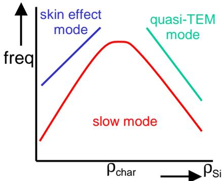
**Figure 9: Overview of the three wave propagation modes that can occur in a Si-SiO<sub>2</sub> system depending on the Si-substrate resistivity.**
