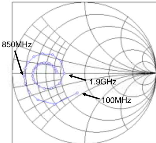
**Figure 10: Smith card with S11 of a 4mm long open microstrip. Already below 1 GHz,  $\frac{1}{4}$  lambda is achieved (real impedance).**
