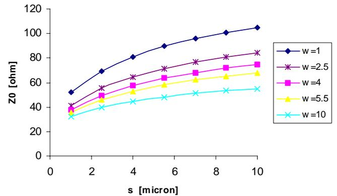
**Figure 6: Odd mode characteristic impedance of metal 5 coplanar striplines above unshielded epi (no M1 shield).**
