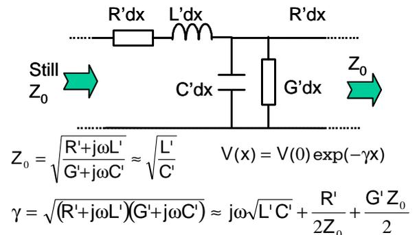
**Figure 1: Distributed circuit element model for a transmission line section and the resulting equations for characteristic impedance and propagation constant. The approximate formulas only hold for frequencies well above f-RC-LC-takeover.**
