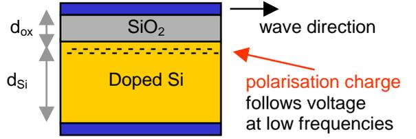
**Figure 8: Si-SiO2 sandwich used as dielectric. L' is determined by  $d_{ox} + d_{Si}$ , while C' is determined by  $d_{ox}$ . As a result the propagation velocity can be much lower than in TEM-mode.**
