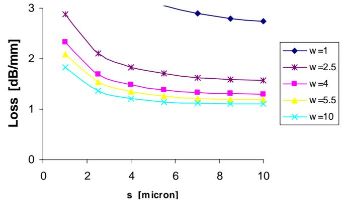
**Figure 5: Loss in dB/mm of metal 5 coplanar striplines above a metal 1 shield.**
