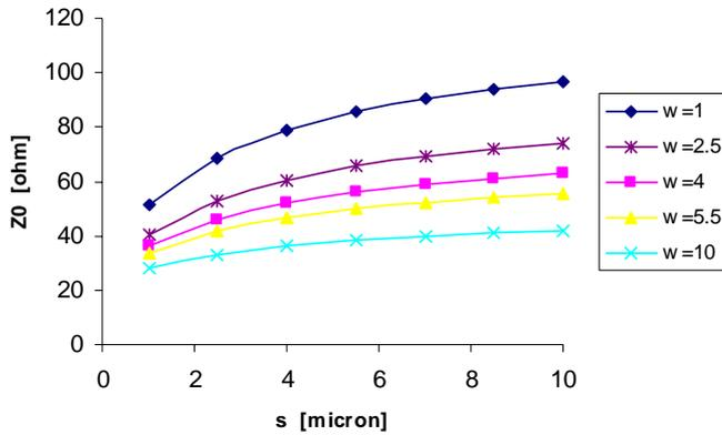
**Figure 4: Odd mode characteristic impedance of metal 5 coplanar striplines above a metal 1 ground shield as a function of separation distance  $s$  for various strip widths  $w$ .**
