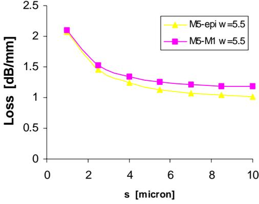
**Figure 7: Detailed comparison of the loss of M5 coplanar strips above a metal 1 ground shield and unshielded epi-layer.**
