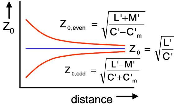
**Figure 2: Characteristic Impedance of coupled lines under Odd mode and even mode drive conditions. For large separation distance the coupling is negligible, and the impedance of a single line is found.**
