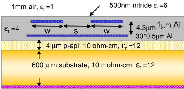
**Figure 3: Coplanar striplines in Metal 5 above a Metal 1 groundplane. M1 shield the substrate from the lines.**
