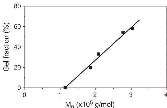
Fig. 1. Effect of PTMC molecular weight on the gel fraction after gamma-irradiation at 25 kGy.
