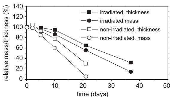
Fig. 2. *In vivo* degradation of PTMC. The  $M_n$  of nonirradiated PTMC is 320 kg/mol, the  $M_n$  of the irradiated PTMC was 480 kg/mol before irradiation.
