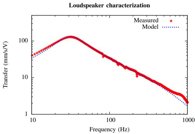
Fig. 2. Comparing model and LDV measurements of the loudspeaker.
