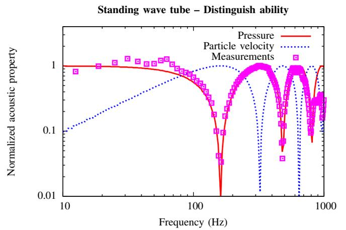
Fig. 6. Determining flow and pressure sensitivity using the standing wave tube.
