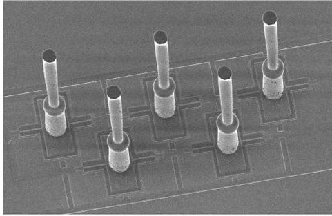
Fig. 1. MEMS hair flow sensors.
