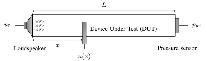
Fig. 5. Schematic of a standing wave tube.
