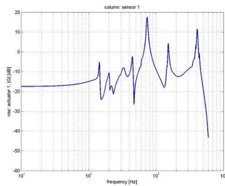
Figure 8. Secondary path transfer function magnitude (actuator 1, sensor 1).
