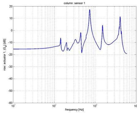
Figure 11. Regularized secondary path minimum-phase transfer function magnitude (actuator 1, sensor 1).
