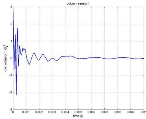
Figure 15. Regularized secondary path minimum-phase inverse impulse response (actuator 1, sensor 1).
