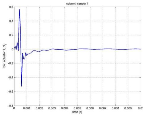
Figure 16. Regularized secondary path all-pass impulse response (actuator 1, sensor 1).
