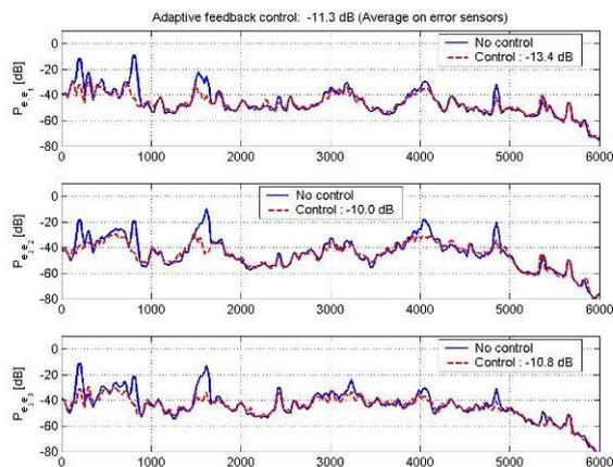
Figure 17. Spectra of the sensor signals, without control and with control using an adaptive feedback algorithm based on Ref. [3].
