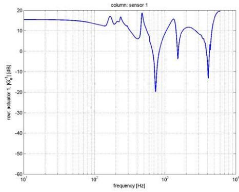
Figure 14. Regularized secondary path minimum-phase inverse transfer function magnitude (actuator 1, sensor 1).
