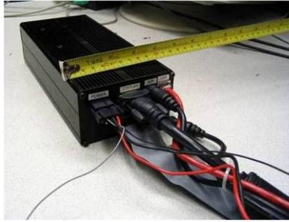
Figure 5. InMAR Control hardware with 16 analog inputs and 16 analog outputs based on an Intel Mobile processor and FPGA.
