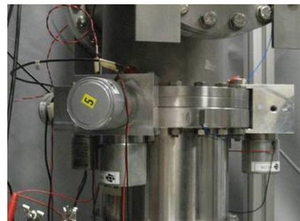
Figure 4. Experimental setup (side view) showing the 3 actuators for the vertical direction and 2 actuators for the horizontal direction.
