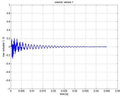
Figure 10. Secondary path impulse response (actuator 1, sensor 1).
