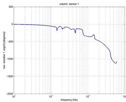
Figure 9. Secondary path transfer function phase (actuator 1, sensor 1).
