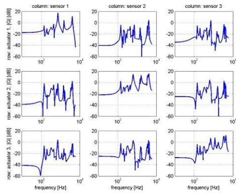
Figure 6. Magnitude of the transfer function between the actuators and the error sensors.
