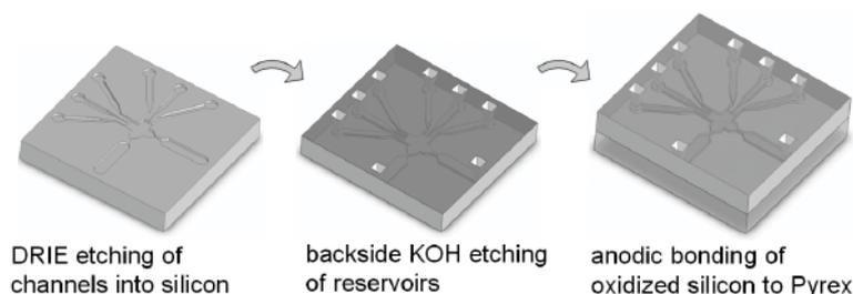
Figure 2. Main fabrication steps for the micro patterning device
