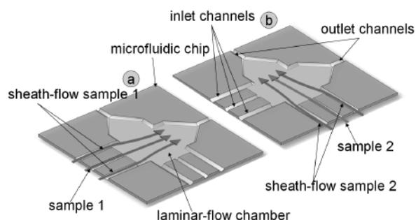
Figure 1. Two perpendicular sample streams operate in terms to immobilize lanes of molecules.
