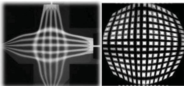
Figure 3. Image overlays visualizing possible array geometry: left: 5x5 streams, right: 13x13 streams with (only the overlapping areas made visible) and a spot size of  $\sim 25 \times 25 \mu\text{m}^2$
