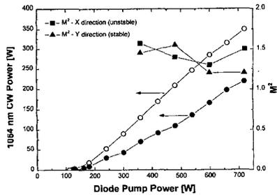
**CTuP4** Fig. 3. Measured output power of a 1 mm thick Nd:YAG slab with a short, stable resonator (open dots) and with the stable-unstable resonator with VRM (filled dots). For the latter resonator, the measured  $M^2$  values in the x-direction (unstable) and the y-direction (stable) are shown as well.
