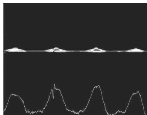
Fig. 2. Broadband  $\text{Ti}^{3+}$  luminescence centered near 760 nm outcoupled from parallel channels of the waveguide array.
