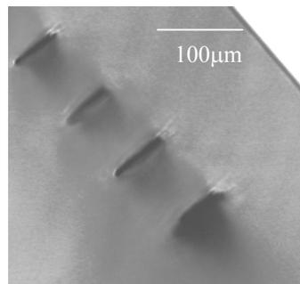
Fig. 1. Microscope image of the end-face of the irradiated  $\text{Ti}^{3+}$ (0.15 at%):sapphire sample.
