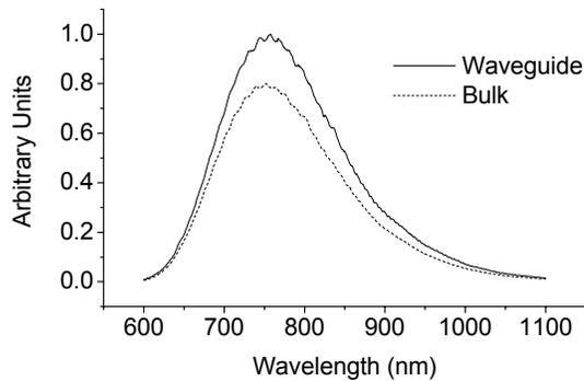
Fig. 3. Fluorescence output signals collected from waveguide and bulk regions of the  $\text{Ti}^{3+}$ (0.21 at%):sapphire sample
