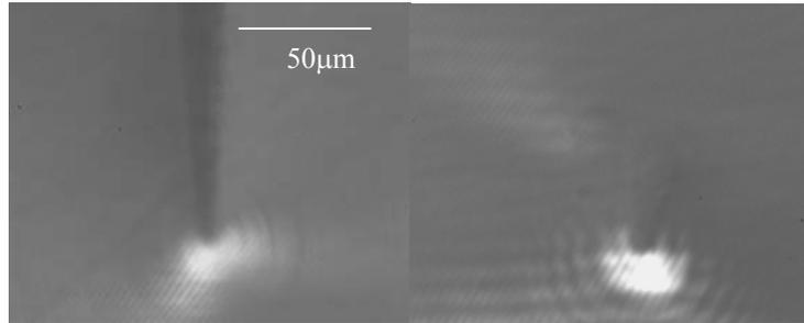
Fig. 2. Mode profiles at 633 nm of two different waveguides written into the bulk of the  $\text{Ti}^{3+}$ (0.21 at%):sapphire sample. (Visible diagonal fringes are due to a detection artifact)
