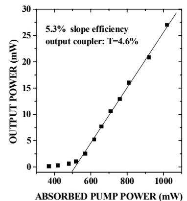
Fig. 3. Output power versus absorbed pump power for a rib waveguide laser with 3.5  $\mu\text{m}$  height and 10  $\mu\text{m}$  width.
