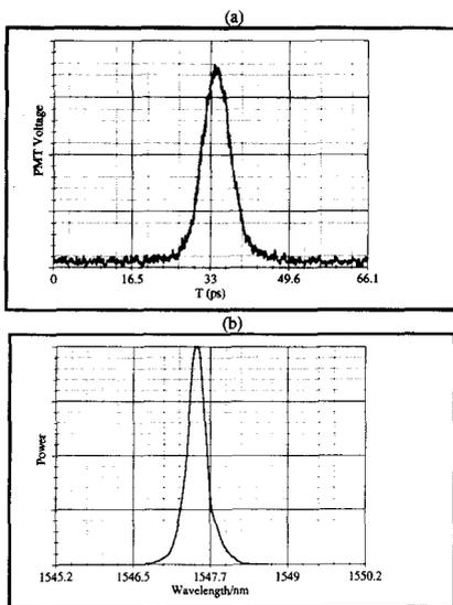
**CFG3 Fig. 3.** (a) Autocorrelation of the switched pulse at the second peak of the double-pass response. The autocorrelation indicates  $\text{sech}^2$  pulses of 6.9 ps (FWHM), compared to launched pulses of 7.2 ps (FWHM). (b) Corresponding spectrum at second switching peak. The spectral width (FWHM) is 0.33 nm.
