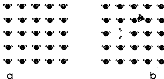
Fig. 3 Energy required to create a cavity-adatom pair on an unreconstructed {001} face in the diamond lattice. \Delta E = 0
