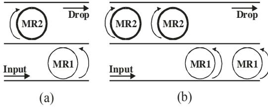
Fig. 1. First (a) and second order (b) wavelength selective switch, MR1: fixed wavelength MR; MR2: tunable MR
