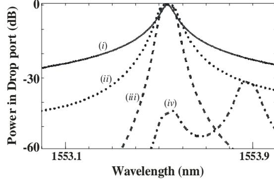
Fig. 2 Response of a MR based switch (i): response of the first stage in Fig. 1.a; (ii): response of the first stage in Fig. 1.b; (iii): response of complete switch in Fig. 1.b in ON-state; (iv): idem in OFF-state.
