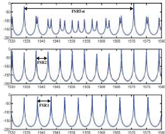
Figure 3. FSR of total switch; constructed of the two separate stages, FSR1 = 4 nm, FSR2=4.5 nm, FSRtot = 36 nm.
