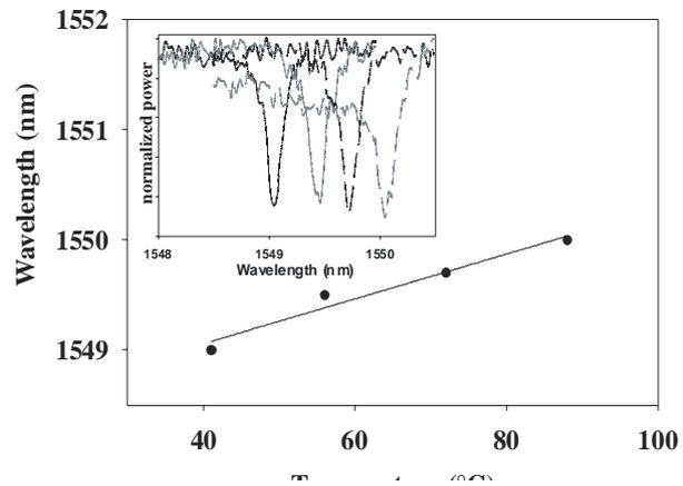
Fig. 4. Thermal dependency of trough- port response of a MR;  $\partial\lambda/\partial T \approx 20$  pm/°C; inset: measured wavelength response
