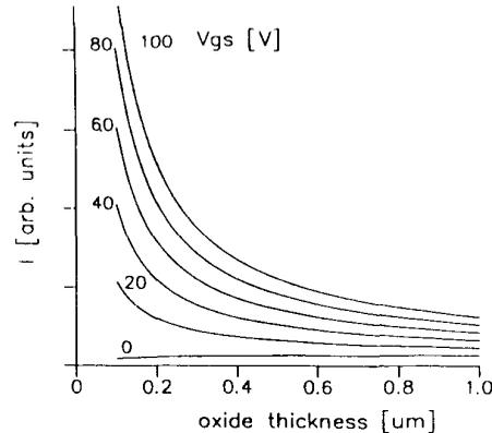
*Figure 2: Theoretical behaviour of the MOSFET with variable insulator thickness.*
