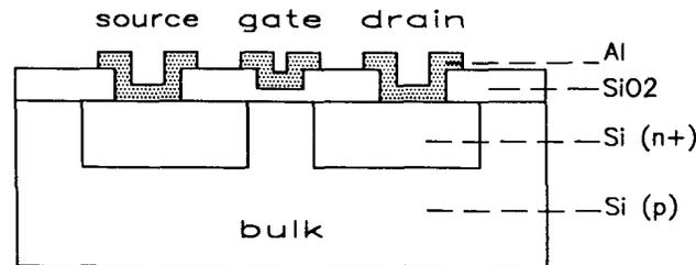
Figure 1: Cross section of the MOS transistor.
