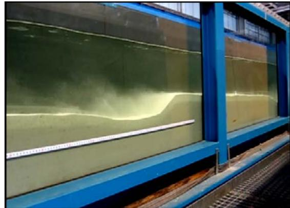
Figure 1. Side view of the flume with fully developed dunes in equilibrium
