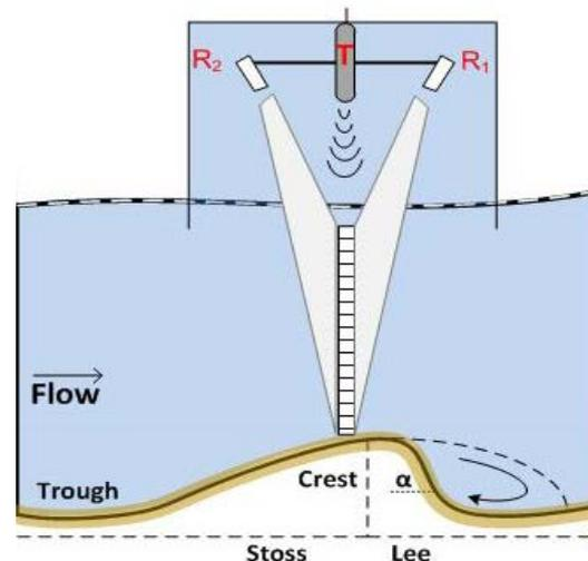
Figure 2. ACVP fixed in a PVC box filled with water (not on scale) and positioned just below the water surface
