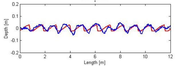
Figure 1. Predicted dune profiles. Red line represents the parameterized dune model, blue line the CA model, flow direction from left to right.
