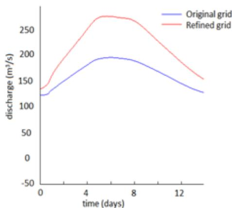
Figure 4. Discharge in side channel at Afferden and Deest for original and refined grid.
