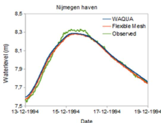
Figure 2. Observed and modeled water levels at location Nijmegen haven for the low discharges in 1994.
