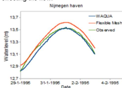
Figure 1. Observed and modeled water levels at location Nijmegen haven for the high discharges of 1995.
