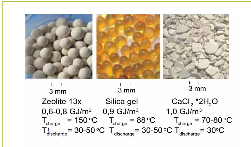
Figure 3: Possible candidates for 1 kW reactor vessel [1].
