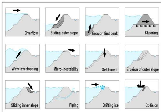
Fig. 1 Failure mechanisms of embankments (TAW 1998)
