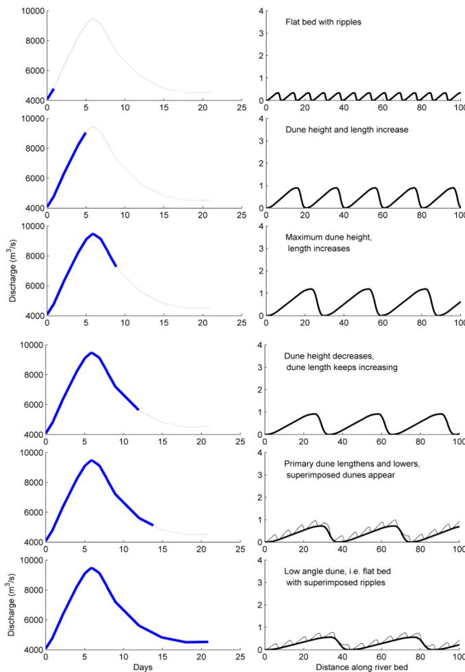
**Figure 2** Proposed model of bed form evolution under varying discharge in flume and field. Left plots: discharge wave of 1995. The right plots illustrate dune development, based on dune height and lengths as observed in the Rhine in 1995 (data from Wilbers and Ten Brinke 2003)
