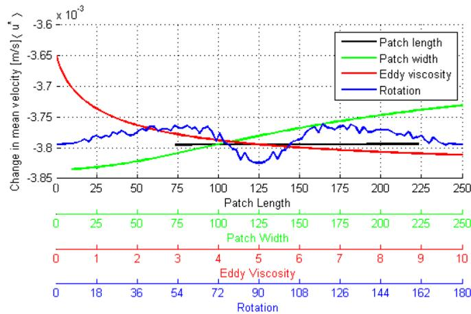
**Figure 7** Influence of patch length, channel width, eddy viscosity and counter clockwise rotation on the mean flow velocity in the channel of a roughness patch as visualized in Fig. 1.
