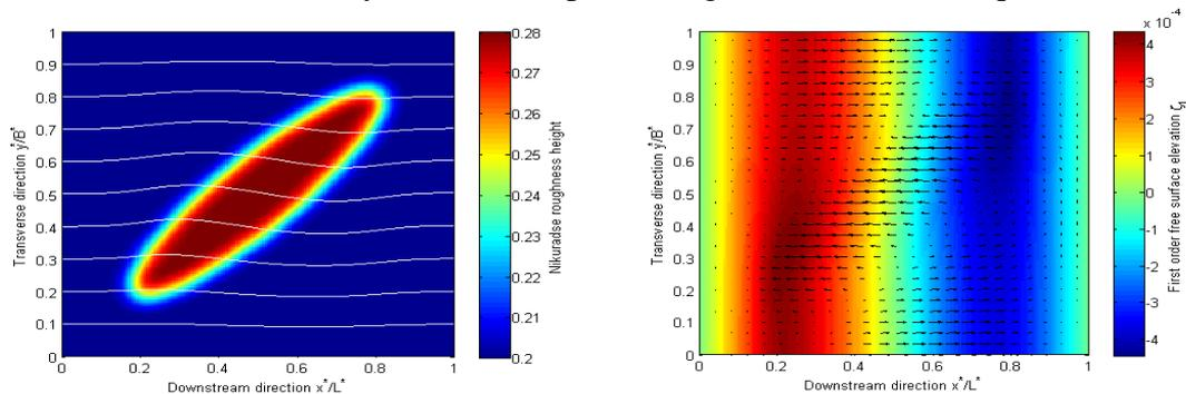
**Figure 6** (Left) shows the roughness patch at a 45° counter clockwise rotation on a floodplain along with exaggerated resulting streamlines of the flow; (right) shows the first order response to this patch. The first order response leads to a spatially invariant response in the second order.
