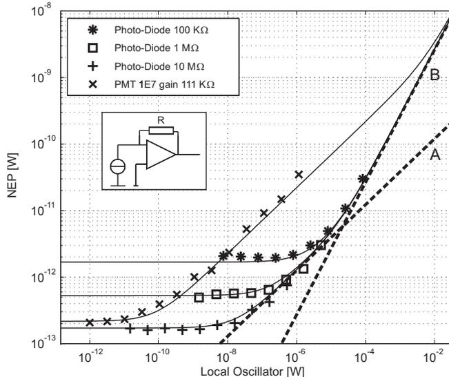
Figure 4. Noise as a function of local oscillator power. The noise is expressed in Noise Equivalent Power (NEP), Root Mean Square (rms) in 1.58 Hz bandwidth so that all lines can be compared directly. The dashed lines A and B have a slope of 1/2, 1 respectively. Continuous lines are a simulation, symbols represent measured data. Inset shows the detector electronics.
