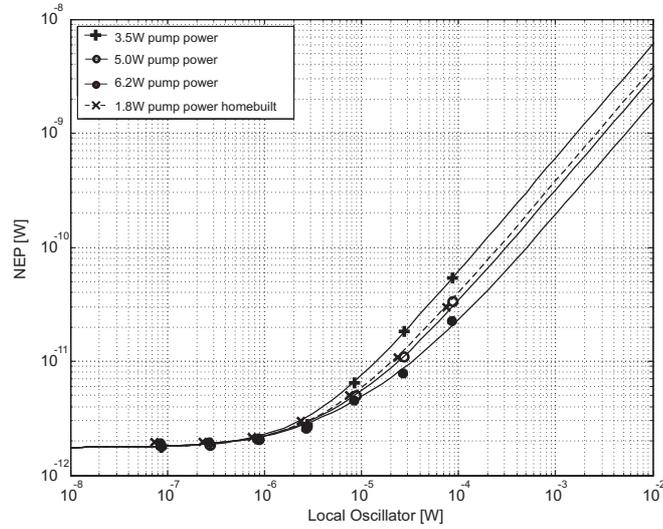
Figure 6. Noise (NEP,  $R=100\text{ k}\Omega$ ,  $BW=1.58\text{ Hz}$ ) for different pump powers (as measured outside the OPO). Combination of Coherent Paladin pump laser and APE Levante Emerald OPO. The dashed line shows the amplitude fluctuations for the homebuilt OPO.
