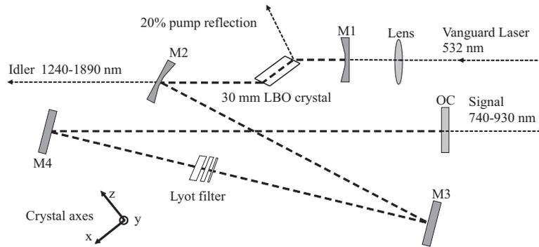
Figure 1. Schematic of the OPO. The resonator consists of a 30mm long Brewster-angled LBO crystal inside a temperature controlled oven, two concave mirrors, M1 (100mm ROC) and M2 (250mm ROC), two plane mirrors M3, M4 and a 6% output coupler (OC). A 200mm lens focuses the 532nm pump beam in the LBO crystal.
