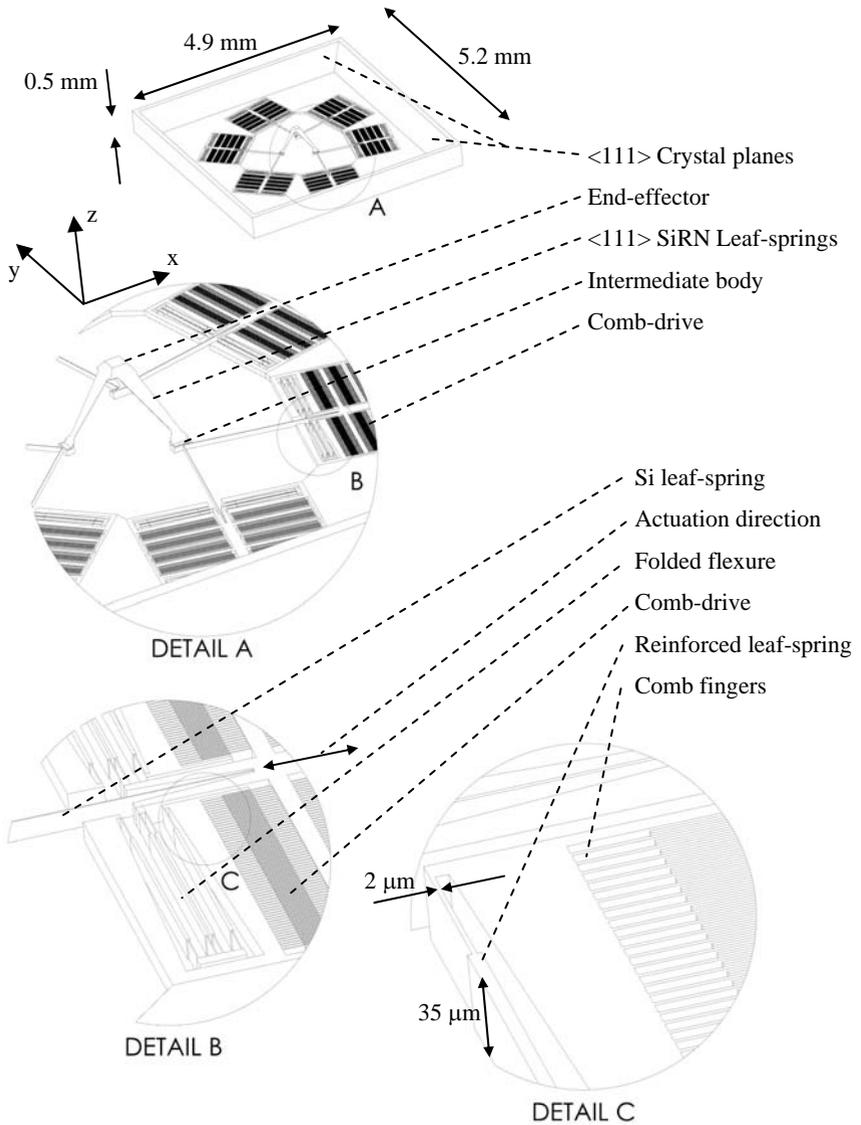
Figure 1: 3D CAD drawings of the MEMS 6 Degrees-of-freedom parallel kinematic precision micro manipulator
