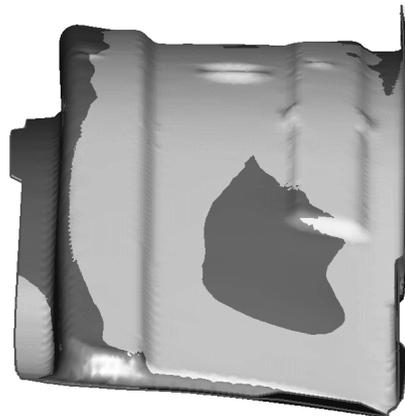
**Figure 2.:** Part geometry after springback (light grey) and after application of the smooth displacement field (dark grey) (exaggeration factor 5)
