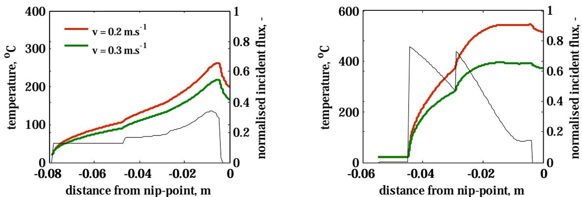
**Figure 6** Incident laser angle  $\alpha$  of  $11^\circ$  Left: substrate surface temperature for two different placement velocities. Right: Tape surface temperature. The thin black lines show the incident heat flux distribution.
