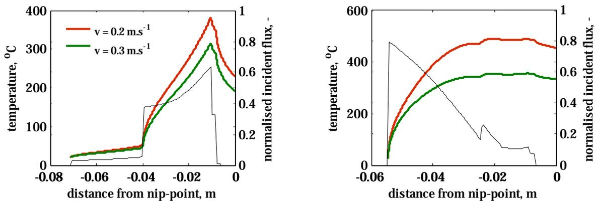
**Figure 5** Incident laser angle  $\alpha$  of  $22^\circ$  Left: substrate surface temperature for two different placement velocities. Right: Tape surface temperature. The thin black lines show the incident heat flux distribution.
