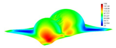
Fig. 1 Enclosed fibre angle for the FEM drape simulation of a double hemisphere geometry (from [1]).
