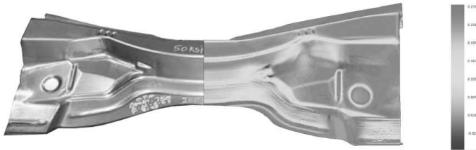
Fig. 3: Automotive underbody cross member - Numisheet'05 benchmark #2
