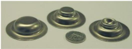
Figure 2: Example parts produced of metastable steels.
