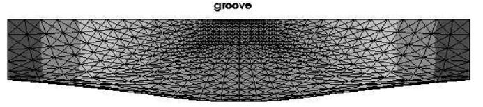
Figure 2: Volume controlled analysis of tube expansion.
