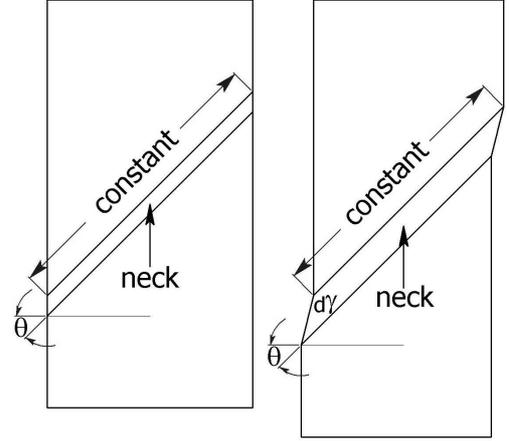
Figure 3: Sheet deformation according to the Hill criterion.
