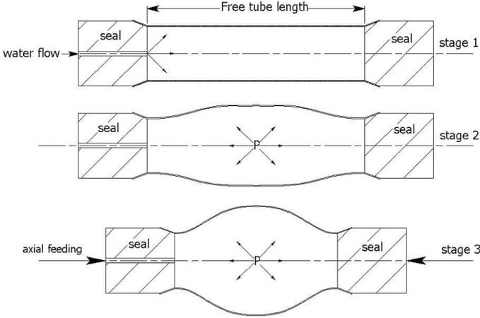
Figure 1: Free expansion test with axial feeding.
