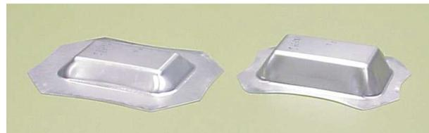
**Figure 8:** Deepest 6016-T4 product at RT (left) and at 250 °C (right)
