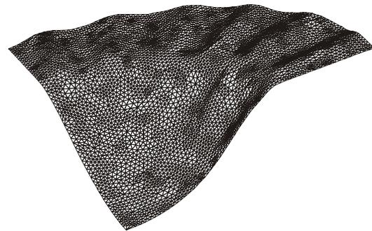
Figure 2. Final mesh (Wrinkling with contact).
