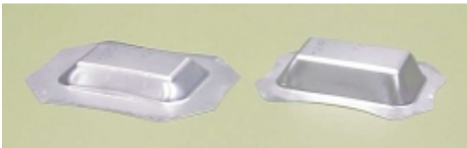
Figure 7: Deepest conical product of 6016-T4 aluminium drawn at RT (left) and at 250°C (right)
