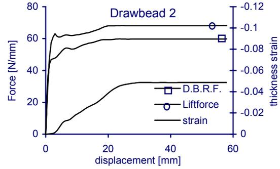
Figure 6. D.B.R.F., lift force and plastic thickness strain for both drawbeads
