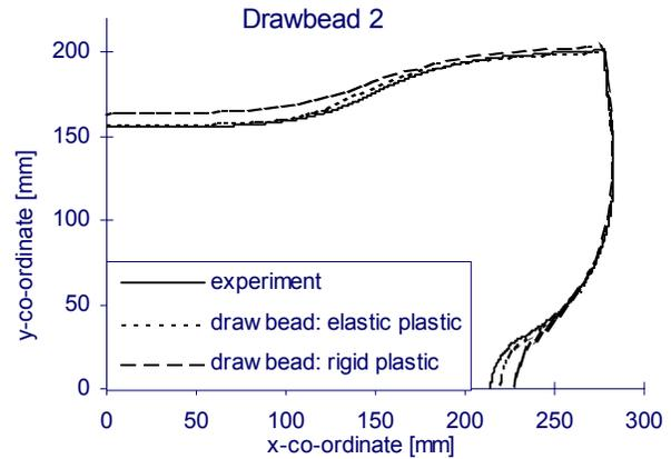
Figure 11. Flange shapes, obtained by using drawbead 2, determined with different material models
