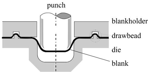
Figure 1. Deep drawing scheme including drawbeads
