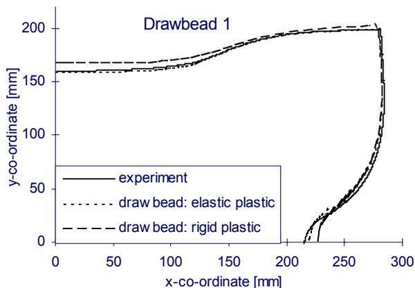
Figure 10. Flange shapes, obtained by using drawbead 1, determined with different material models
