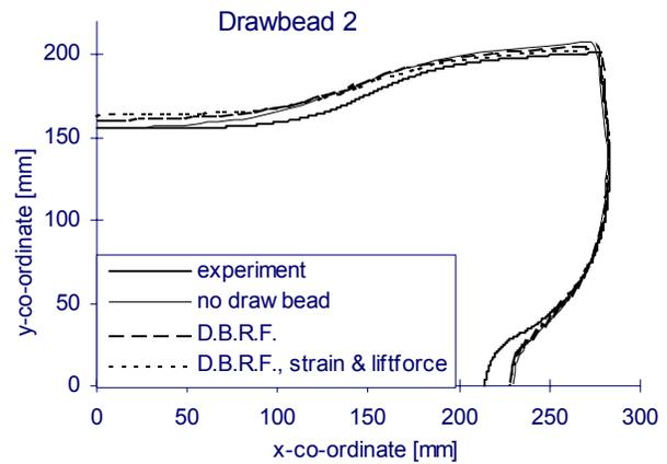
Figure 9. Flange shapes, obtained by using drawbead 2, assuming a rigid plastic material behavior
