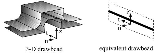
Figure 3. Schematic of a real drawbead and its equivalent representation
