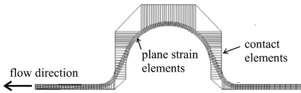
Figure 2. Finite element mesh of a 2D drawbead model
