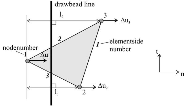
Figure 4. Node and element side numbering
