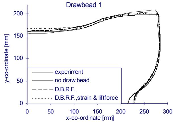
Figure 8. Flange shapes, obtained by using drawbead 1, assuming a rigid plastic material behavior
