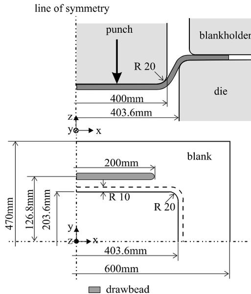
Figure 7. Tool geometry of the rectangular product
