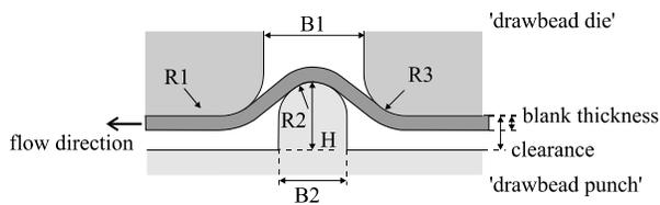
Figure 5. Drawbead geometry
