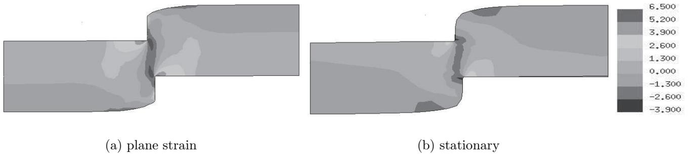
Figure 9: hydrostatic pressure (\*100MPa) at 50% penetration
