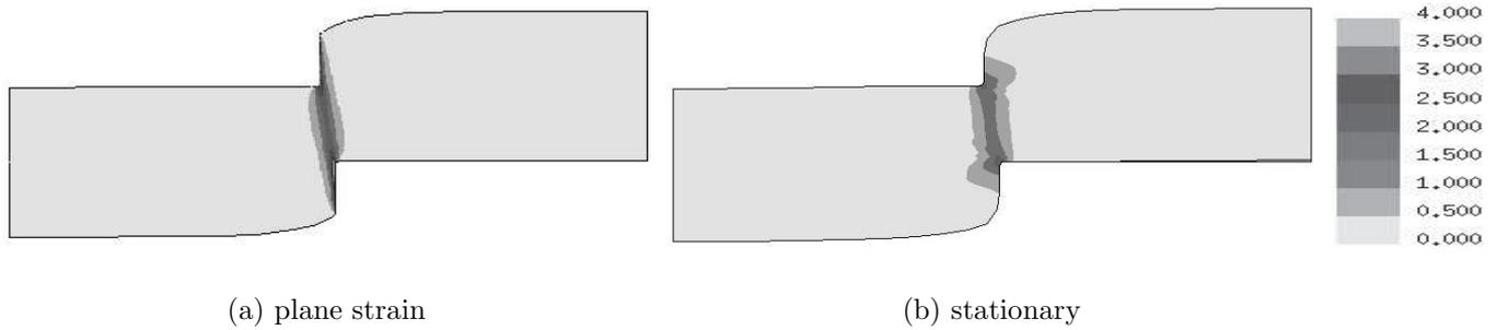
Figure 8: equivalent plastic strain at 50% penetration
