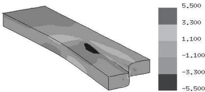
Figure 10: bending stresses:  $\sigma_{xx}$  (\*100MPa)
