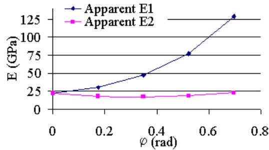
Fig 9: Apparent moduli of skewed fabric
