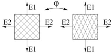
Fig 8: Loading of fabric
