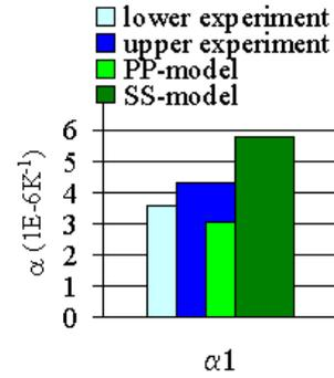
Fig 7: CTE for orthogonal fabric
