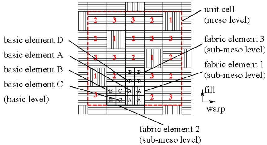
**Fig 1:** Unit cell of Satin 5H weave, with fabric elements 1, 2, 3 and basic elements A,B,C,D
