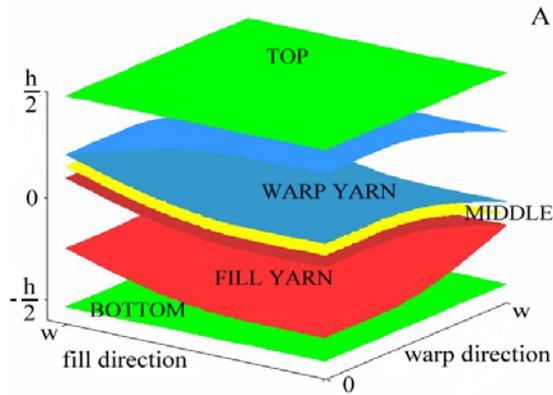
Fig 4<sup>a</sup>: Basic element A
