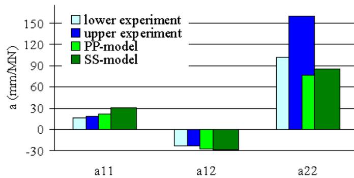
Fig 6<sup>c</sup>: Intermediate skew fabric results ( $a_{11}$ ,  $a_{12}$  and  $a_{66}$ )
