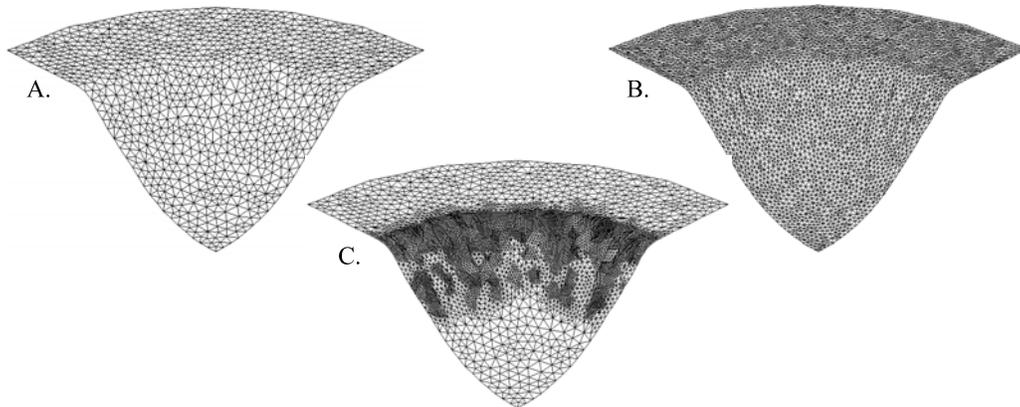
Figure 2. Deformed meshes (A: Coarse mesh - B: Fine mesh - C: Refined mesh)
