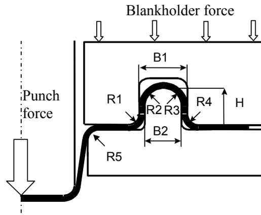
Figure 2. Drawbead test equipment
