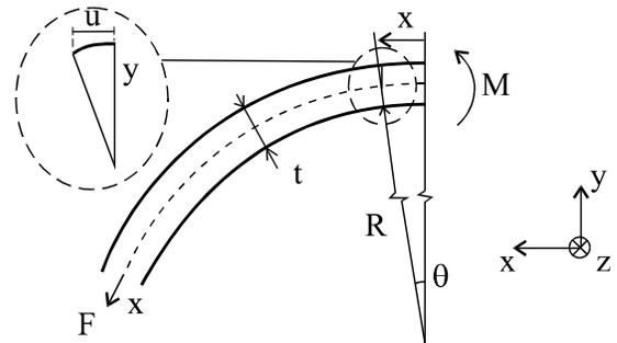
Figure 5. Principle outline for calculation of bending force
