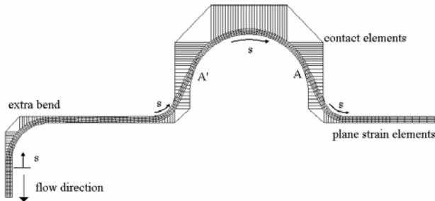
Figure 1. Finite element mesh of the 2D drawbead model
