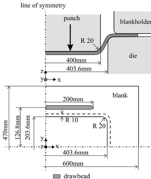
Figure 10. Tool geometry of the rectangular product
