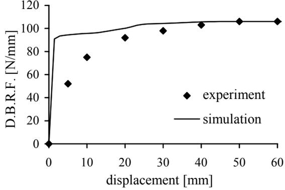
Figure 3. Drawbead restraining force
