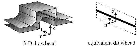
Figure 6. Schematic of a real drawbead and its equivalent representation
