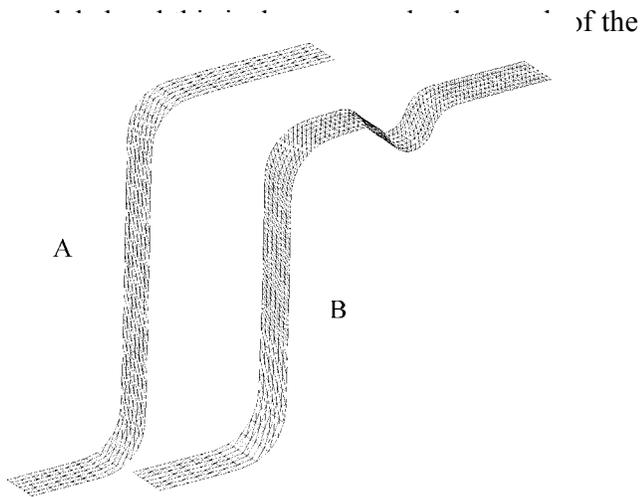
Figure 7 Finite element models of strip drawing with real drawbead (B) and with an equivalent drawbead (A)
