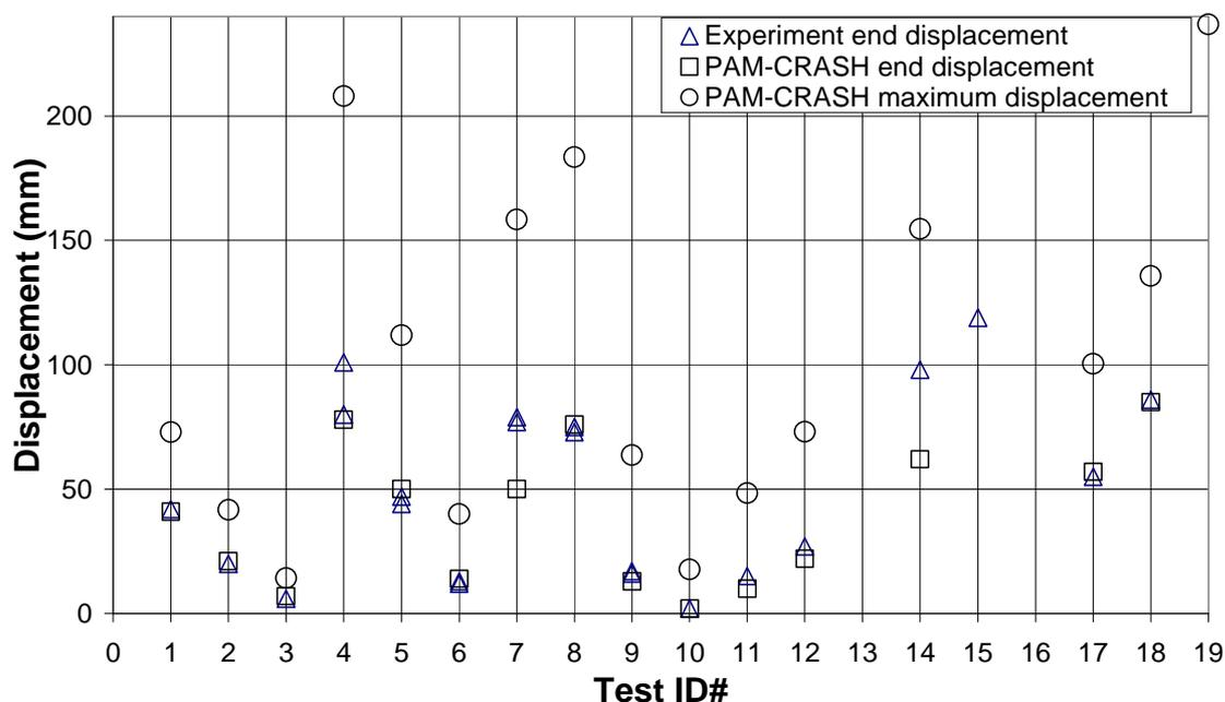
Figure 5 Comparison of displacements from experiments and numerical simulations. The measured and simulated end displacements are close to each other. The maximum displacement shows a similar trend as the end displacement. Prediction of one displacement from the other is therefore possible.
