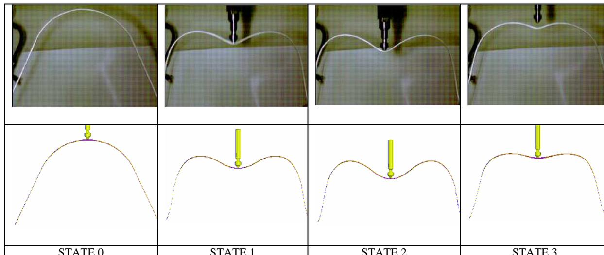
Figure 4 High-speed camera pictures (top) and simulation results (bottom) at different states.
