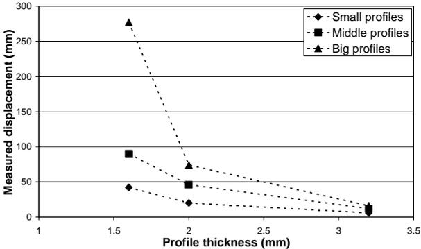
Figure 3 Relations between profile thickness and measured end-displacement for three different sized profiles. The remaining end displacement increases for larger profiles with similar thickness. With thick profiles, end displacement depends less on the profile size.
