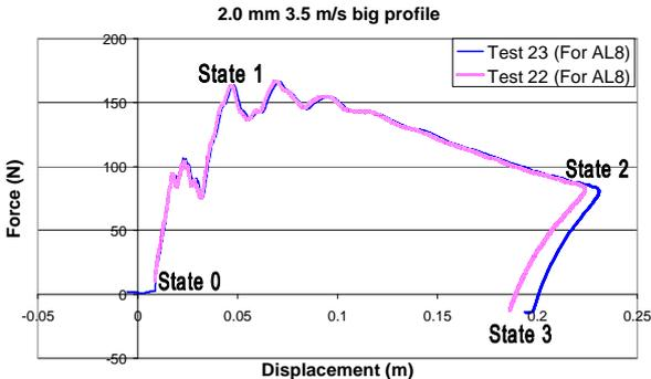
Figure 2 Repeatability of force-displacement curves for two impact tests on identical profiles.
