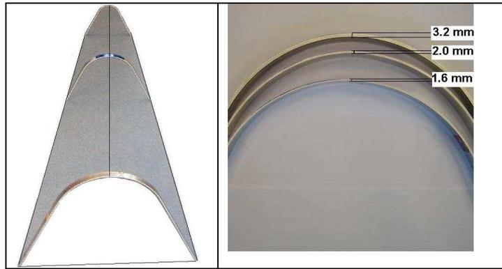
Figure 1 On the left, three different sized two-dimensional profiles are shown. They are chosen at the root, the middle and the tip of the leading edge. Typical length of the leading edge is 6 meters. On the right, three different thicknesses are shown. These are typical thicknesses found in leading edges.
