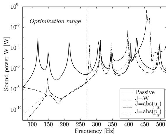
Figure 4: Comparison of radiated sound power reduction for different error criteria.
