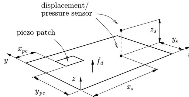
Figure 2: Clamped rectangular plate with one piezoelectric patch.
