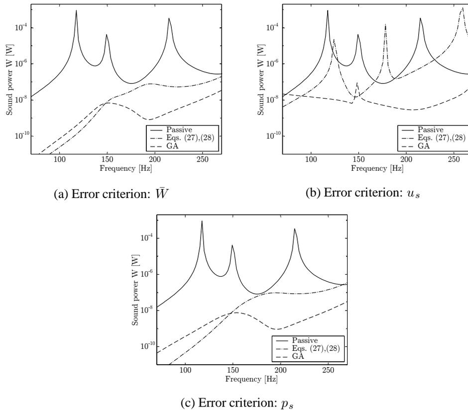
Figure 3: Comparison of optimal configurations for different error criteria: (a) radiated sound power  $\bar{W}$ , (b) out-of-plane displacement  $u_s$ , and, (c) near-field acoustic pressure  $p_s$ .
