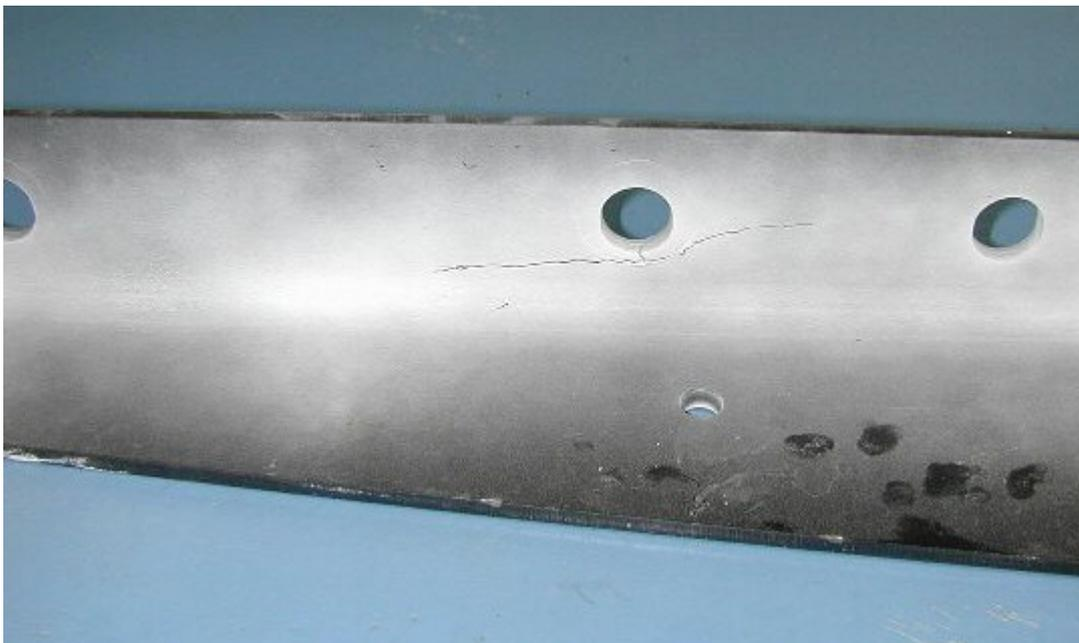
**Figure 7: Fatigue failure at the hot-spot during testing**
