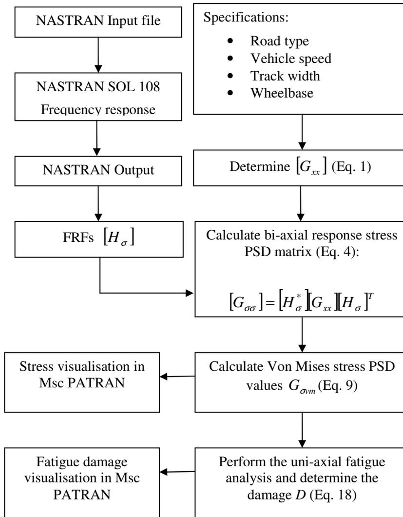
Figure 4: Implementation of the method for fatigue analysis
