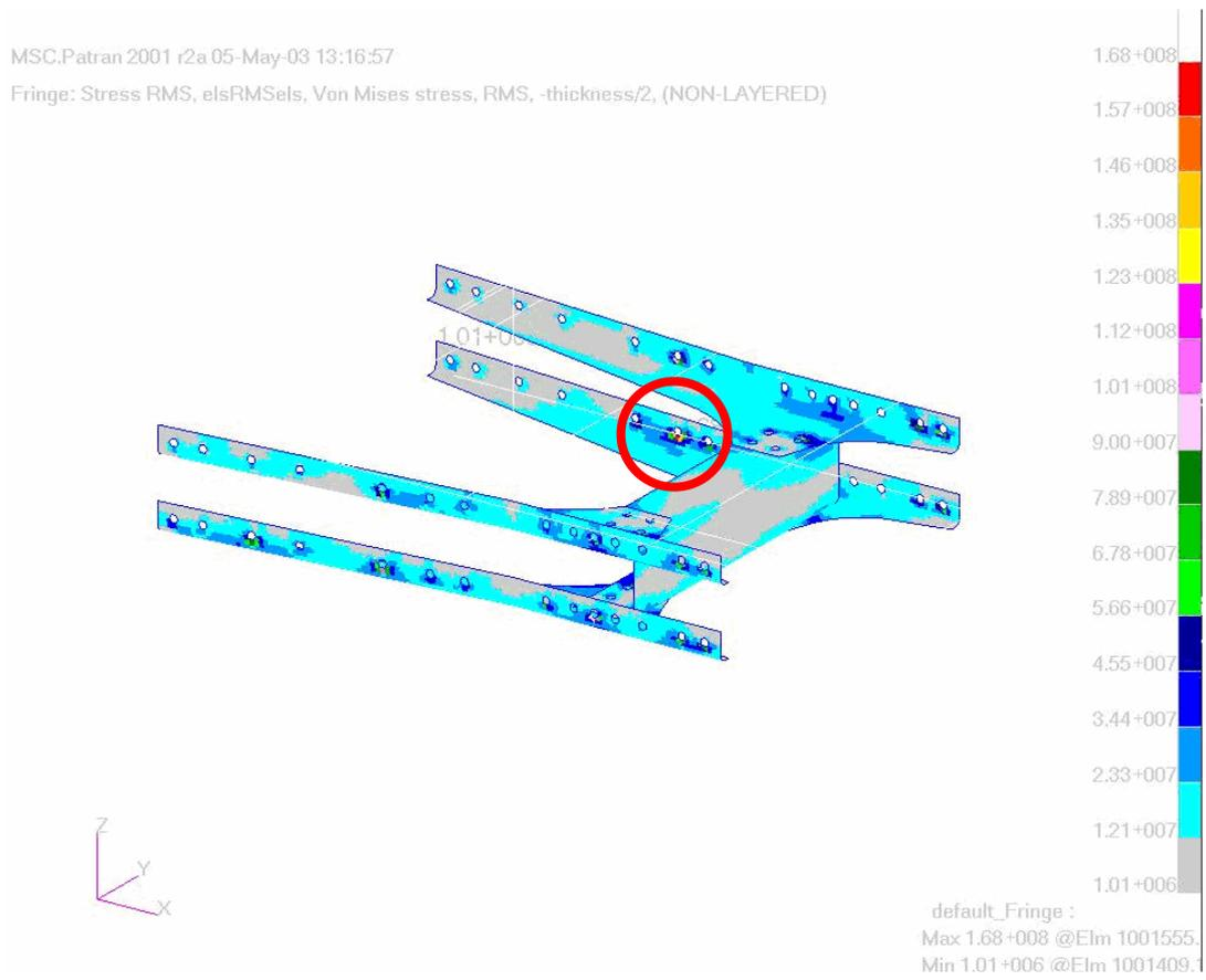
**Figure 6: RMS values of the Von Mises stress**
