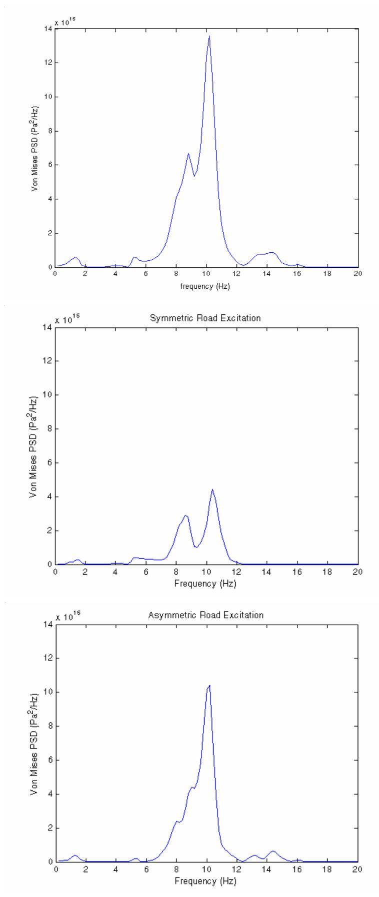
**Figure 8: Von Mises stress PSDs at the hot-spot**
