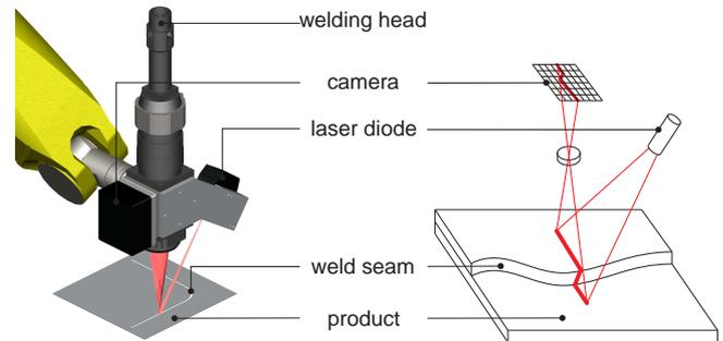
Figure 2 : Seam tracking sensor
