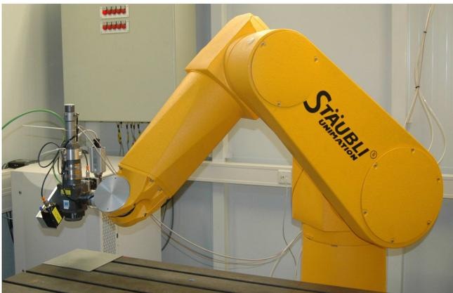
Figure 1 : The six-axes industrial Staubli RX130 robot
