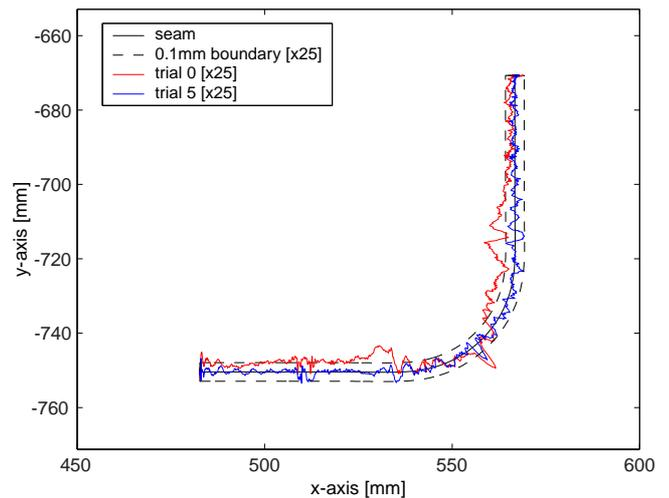
Figure 3 : Tracking error perpendicular to weld seam
