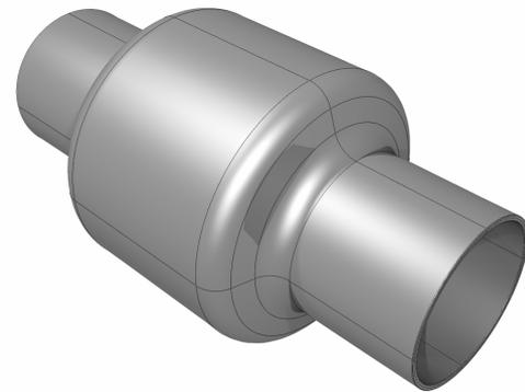
Figure 2: Hydroformed part used as Demonstration of Concept
