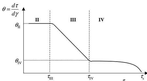
Figure 2 : Strain hardening versus flow stress
