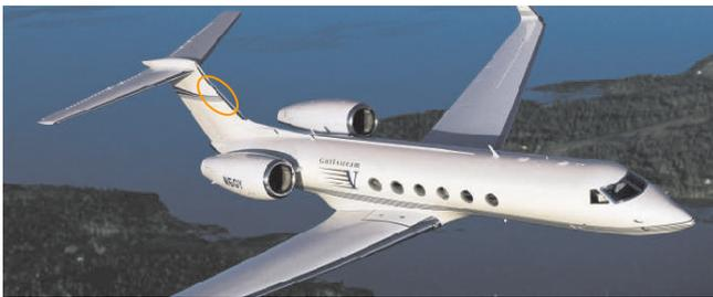
Figure 1 : Leading edge of the tail of an airplane
