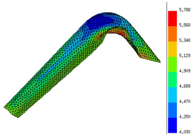
Figure 3: Thickness after first draw [mm].
