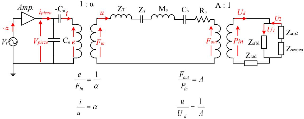
Figure 9: Lumped equivalent electrical circuit of the perforated honey-comb loudspeaker driven by one stack piezoelectric actuator.
