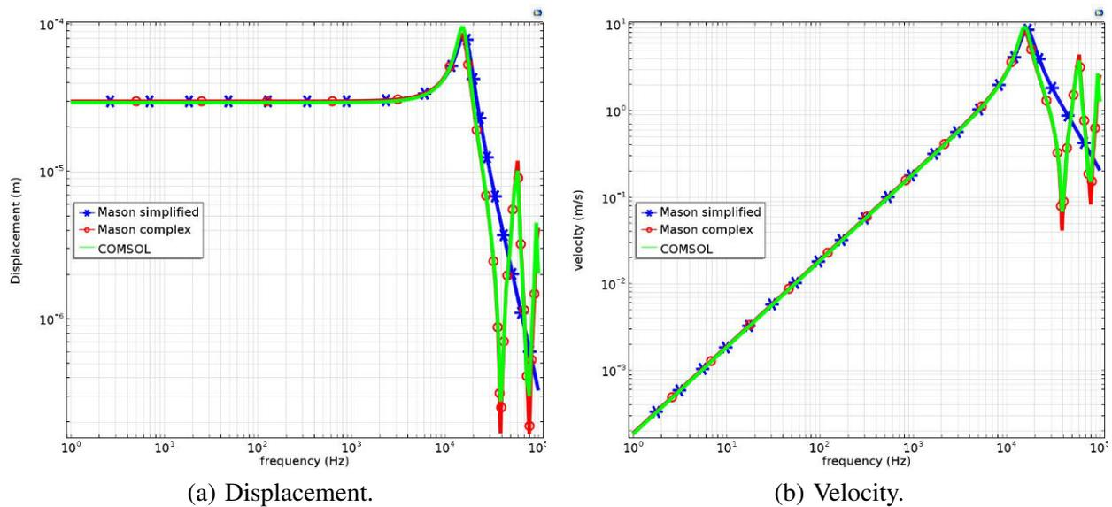
Figure 3: Mechanical behavior of a single piezoelectric actuator in the free vibration regime with one end clamped
