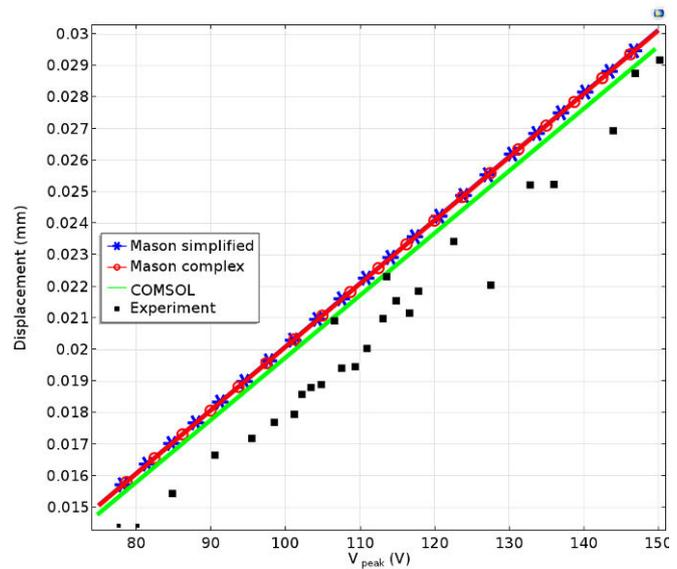
(b) Characteristics diagram of a single piezoelectric actuator in the free vibration regime with one end clamped under various applied voltage.
