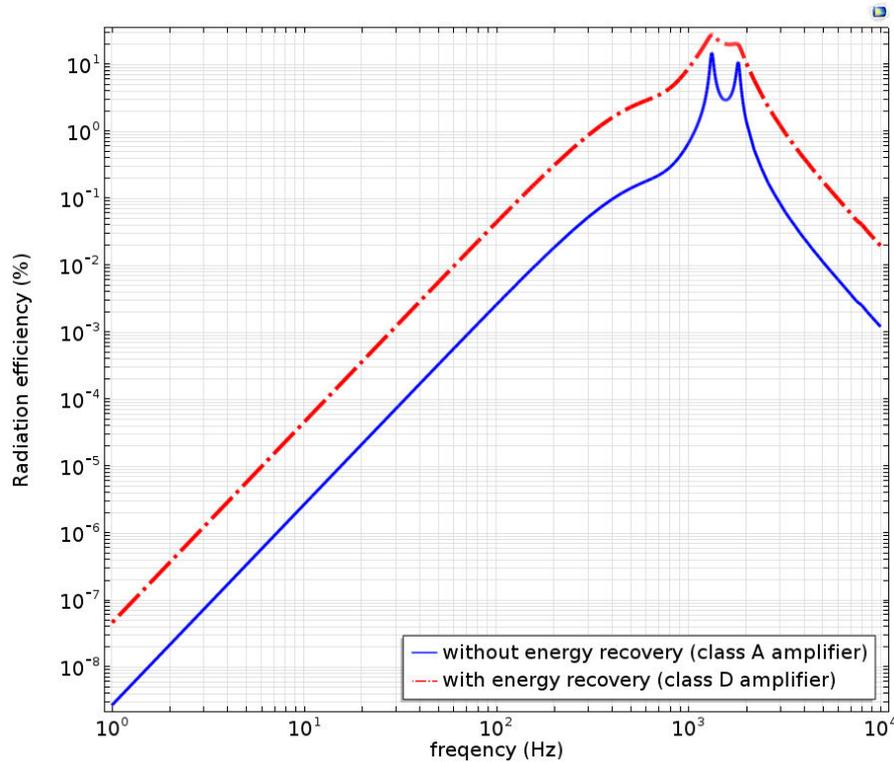
Figure 11: Efficiency of the acoustic source when it is connected to analogue and switching amplifiers.
