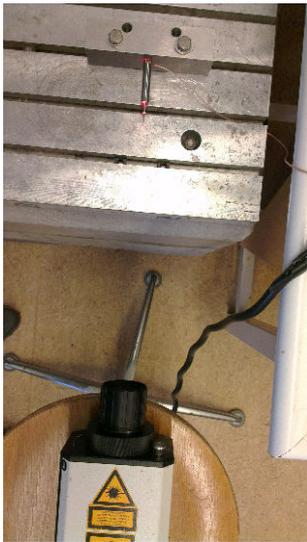
(a) Test setup for measuring the free stroke of the piezoelectric stake actuator with laser.
