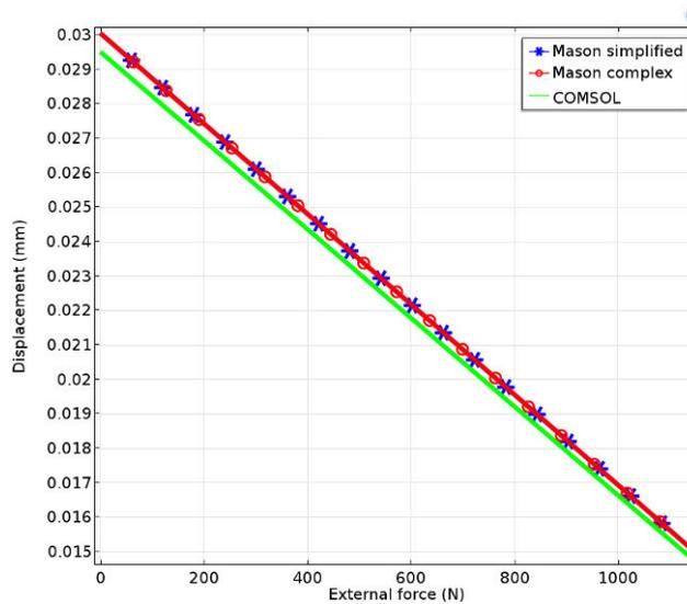
Figure 5: The characteristic diagram of a single piezoelectric stack actuator in semi-blocked regime with one end clamped under various external forces.
