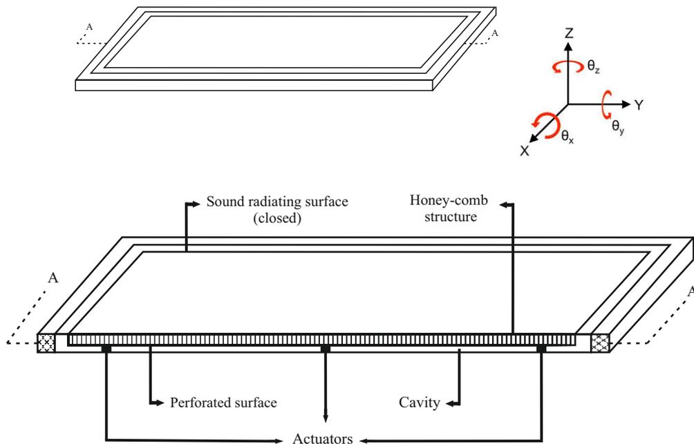
Figure 8: The acoustic source based on a honey-comb structure with A–A cross section view.
