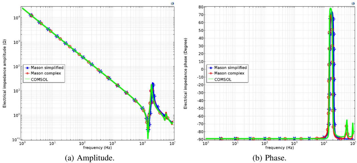
Figure 4: Bode diagram of electrical impedance of a single piezoelectric actuator in the free vibration regime with one end clamped
